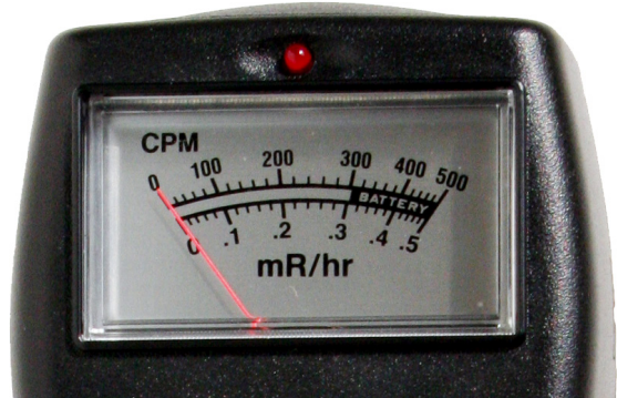
M4 with CPM & mR/hr meter scale
