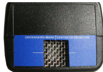
The end window of the M4 and M4EC
